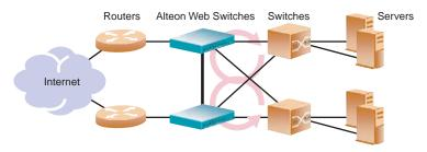
Figure 11-12 Cross-Redundancy Creates Loops, But STP Resolves Them
